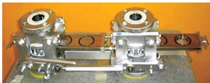
Рис. 4. Twin Lineblind 2" three positions slide
